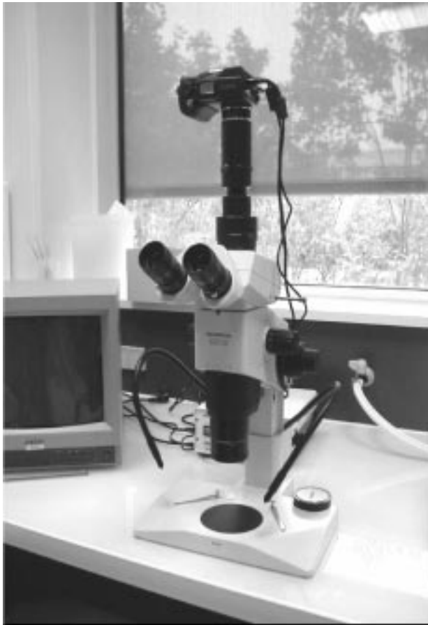
Fig. 9.3 Stereomicroscope for viewing texture defaults.
